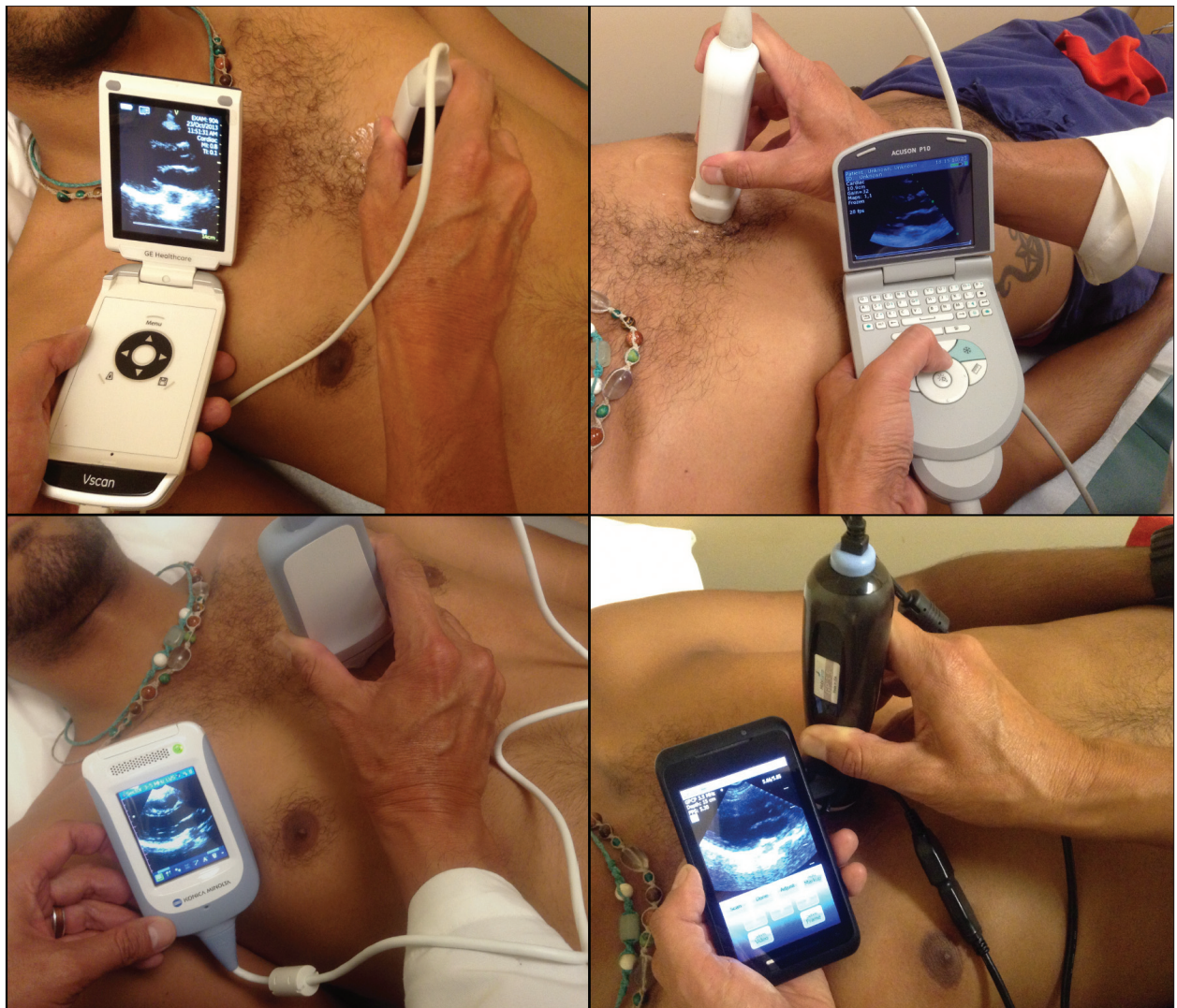
Figure 2. Currently available pocket-sized devices. Top left, Vscan, 1.7–3.8-MHz phased array transducer (GE Healthcare, Wauwatosa, WI; approved 2009). Top right, Acuson P10, 2–4-MHz phased array transducer (Siemens Medical Solutions USA, Inc, Malvern, PA; approved 2007). Bottom left, Sonimage P3, 3–5-MHz mechanical interchangeable transducer (Signostics Ltd, Thebarton, South Australia, Australia; approved 2013). Bottom right, MobiUS SP1, 7.5–12-MHz mechanical interchangeable transducer, smartphone connected (Mobisante, Inc, Redmond, WA; approved 2011).
