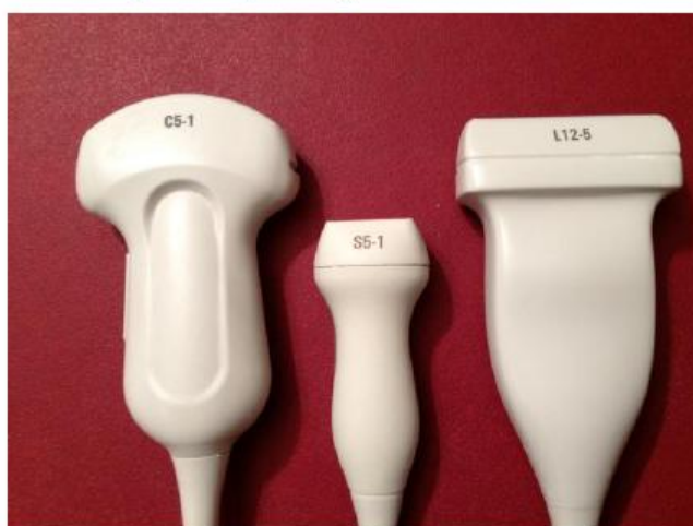
Figure 8 Ultrasound probes for optimal liver investigation: Convex probe (C5-1) is commonly used. Sector probe (S5-1) may be beneficial in obese patients. Linear probe (L12-5) is used to assess the liver surface.
