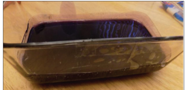
Figure 12. Finished product, with the second tissue layer pressed onto the spine model. No additional adhesive or heating is required.
